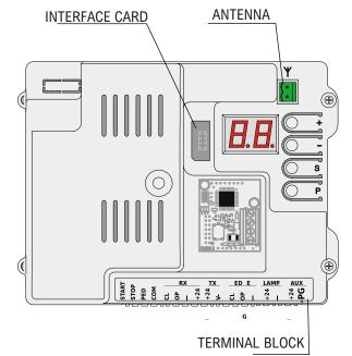
After outlining the wiring plan, proceed to remove the plastic cover: pull out the antenna connector, loose the 2 screws and open the housing. If you decided to drill a hole to let the wires pass through, do it at this stage.
