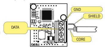
Above a TWINNING card top view showing wirings (a shielded or RG58 cable is required). A small section cable will be sufficient, since it is used just for signal tranfer.
